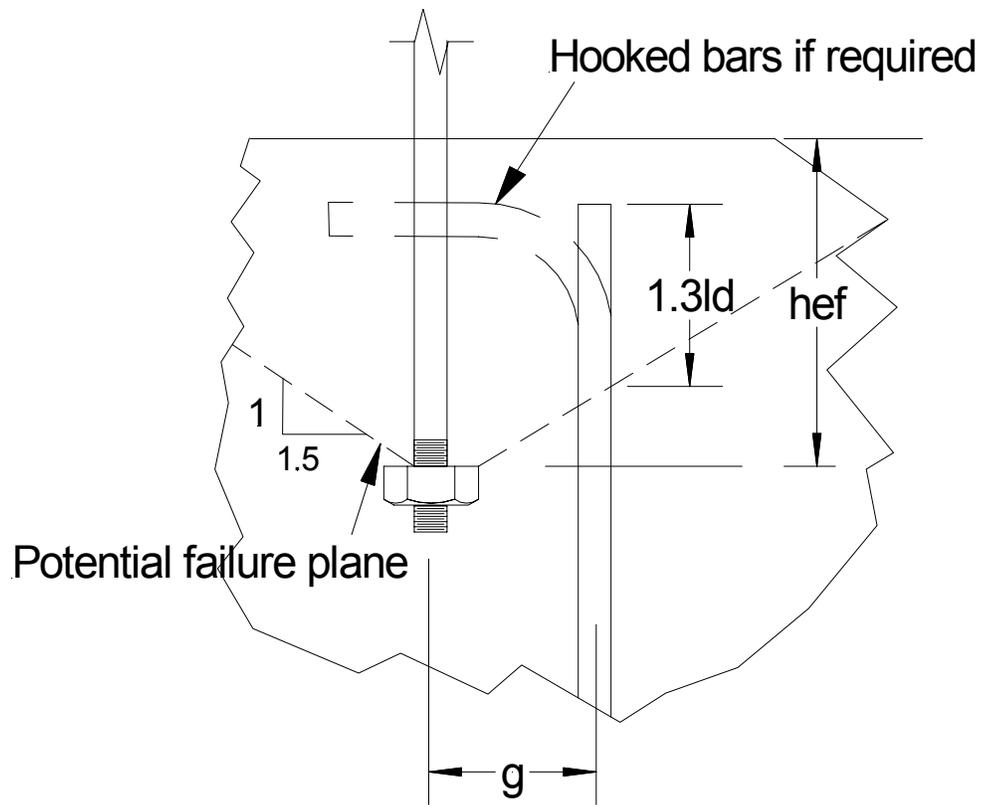
Fig. 5- 2 Development of bar for concrete breakout
