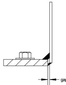
Must build out weld to
